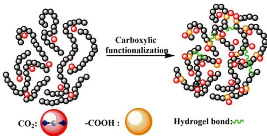
FIGURE 1 | Mechanism by which hydrogel absorbs CO 2 . Reproduced with permission [47]. Copyright 2021, Elsevier. [Color figure can be viewed at wileyonlinelibrary.com ]
