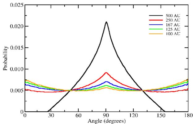
**Figure 4.** Distribution of nanorod filler orientations in the different lattice length at filler concentration equal to 7.2 %volume.
