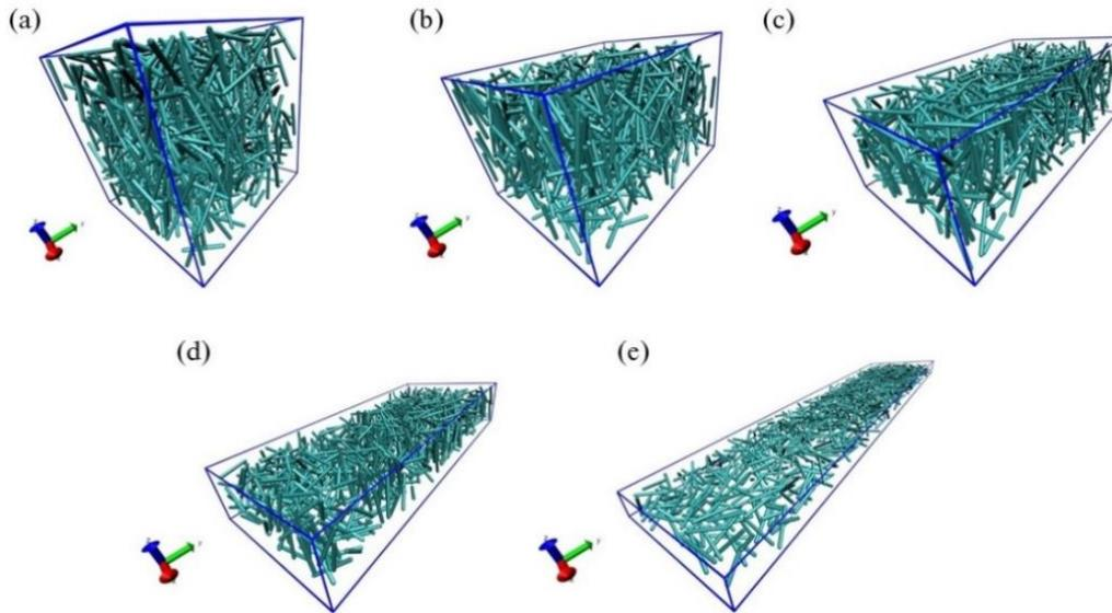
**Figure 1.** The lattice filling with nanorod filler at the lattice height of (a) 100 AU, (b) 80 AU, (c) 60 AU, (d) 40 AU and (e) 20 AU. Visualizations were done by Visual Molecular Dynamics(VMD)[9]
